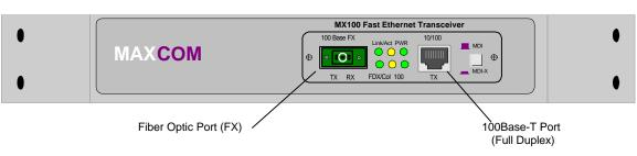
Front Panel - Single Fiber with SC/APC Fiber Optic Connectors
