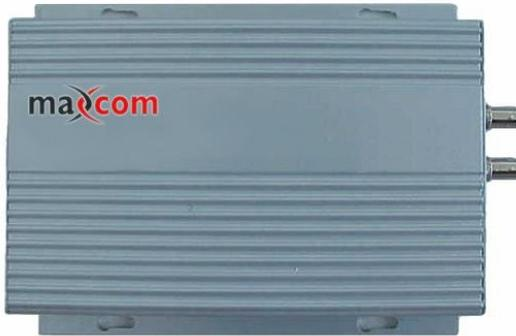
The MX ASI-IP Network Adapter is a special purpose device capable of converting from DVB ASI to IP UDP, which can be used in any ASI (270Mbps) data to IP application.
