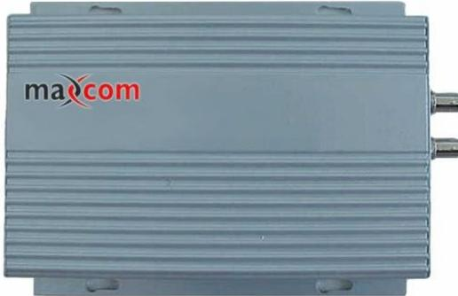
The MX IP-ASI Network Adapter is a special purpose device that converts IP UDP back to DVB ASI. Using in pairs with MX ASI-IP Network Adapter, A DVB ASI stream can be transmitted through Ethernet Networks.
