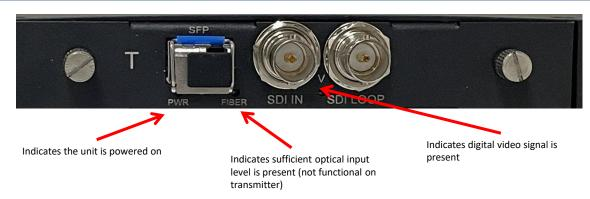
Transmitter will only have optical output when a compliant digital video signal is present (ASI, SDI, SMPT..) Transmitter will have green light "P" when powered on, and green light "V" when video signal is present ("F" light not used on transmitter)
