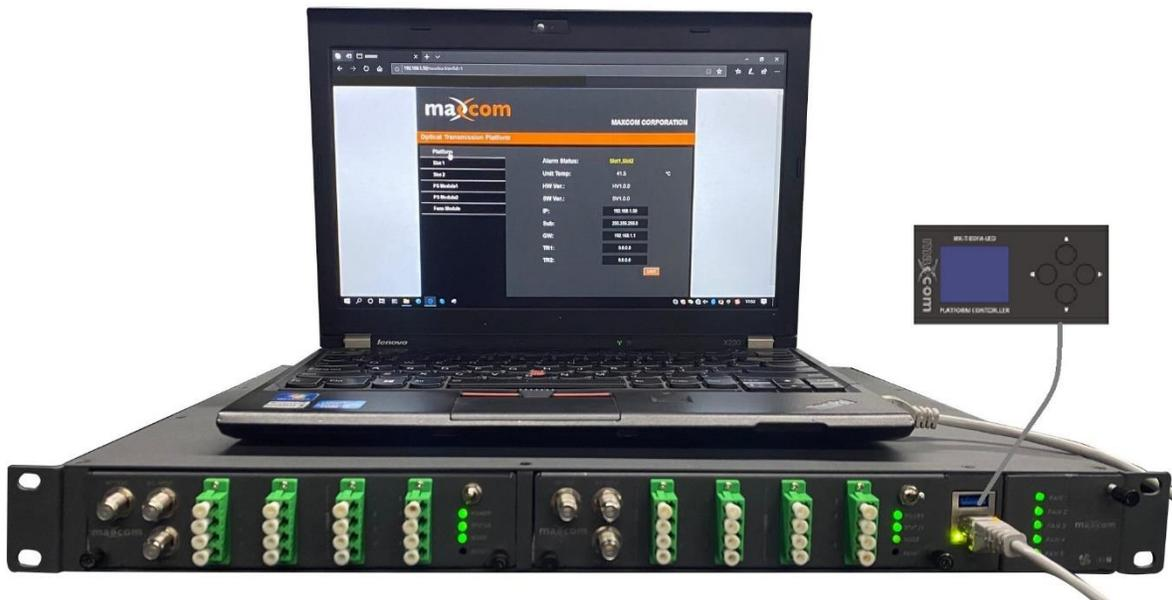
The MX-T-EDFA is a highly integrated, yet simple device specifically designed for Cable Telecommunication Systems deploying RFoG or RF Overlays in the FTTx environment with integrated filters supporting GPON and/or XG(S)PON (10G). Its small size and high density make it the ideal choice, particularly in tightly enclosed environments.
